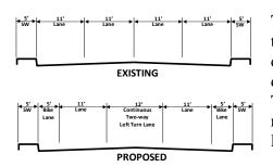
TrafInfo was tasked with conducting a Road Diet study on two existing four lane highways. The study involved a detailed field investigation; development of collision diagrams; and review of research articles in trade journals. TrafInfo developed conceptual plans for a three-lane roadway including a continuous two-way center left turn lane as well as 5-foot bike lanes on either side.
